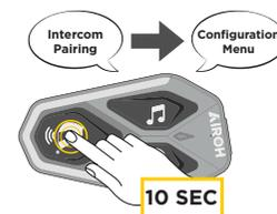
With AWC 4 turned on, press the power button for 10 seconds to enter configuration mode. Do not release the button before the LED turns blue. A confirmation voice prompt will be heard.
